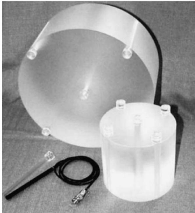
16 cm (HEAD) and 32 cm (BODY) PMMA Phantom with 10cm bar-dosimeter
